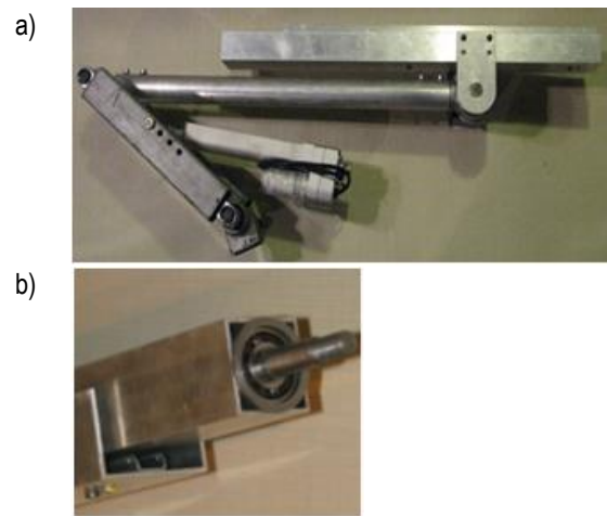
Fig. 7. Selected views of manipulator prototype: a) initial configuration view; b) linear and revolute joints of effector
